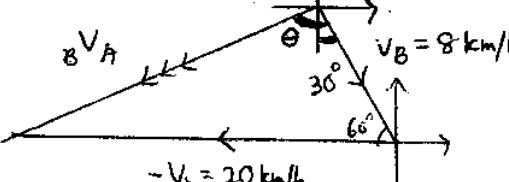
${}_{\text{B}}V_A^2 = 8^2 + 20^2 - 2(8)(20)\cos 60^\circ$ ${}_{\text{B}}V_A^2 = 304 \quad , \quad {}_{\text{B}}V_A = 17.4356 \quad \text{or} \quad {}_{\text{B}}V_A = \sqrt{304}$ <p>The velocity of B relative to A is 17.44 km/h .</p>                                      | D1<br>diagram<br><br>B1                                                             |
